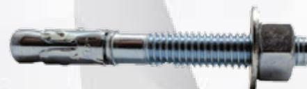
The wedge anchor are fully threaded, torque-controlled, design for consistent performance in cracked and non-cracked concrete base materials including normal weight concrete, sand lightweight concrete deck. Range of size from M8-M16
